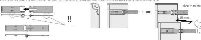
Snap the cover onto the hinges. Close it and secure it using the supplied screws. After the settings and adjustments, fasten the cover using the supplied screws.
